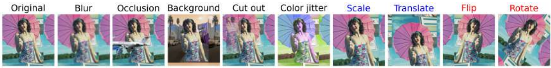
FIGURE 4.7: Augmentations for the Body subnetwork. Black, blue and red labels represent image-variant, location-variant and pose-variant augmentations, respectively.
