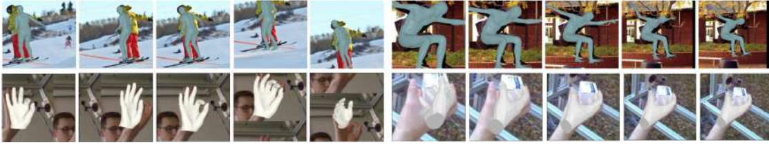
FIGURE 4.3: Sensitivity of existing body and hand models to different alignments (left) and scales (right).
