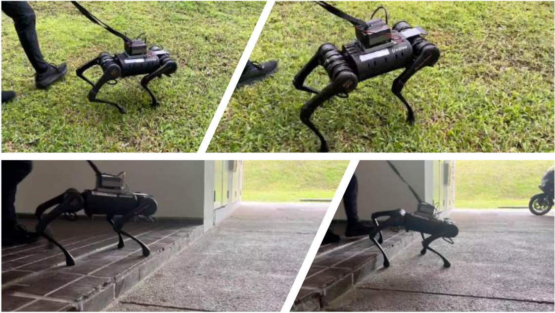
FIGURE 3.8: Deployment in the physical world on Unitree A1 with minimized observations with zero-shot transfer.
