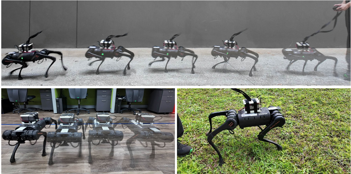
FIGURE 5.4: Footage snapshots showing a single trained ULT policy deployed in the real world with zero-shot transfer on Unitree A1 equipped with Jetson Orin AGX for inference on different terrains with motion in omnidirections.
