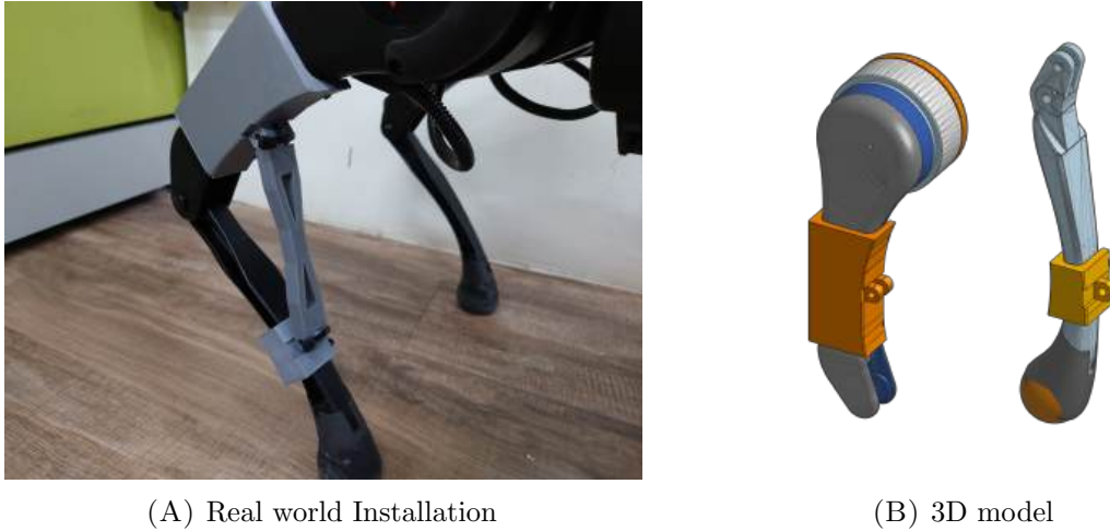
FIGURE 4.3: The 3D-printed joint locking mechanism assembled in the physical device A , containing two mounts for thigh link and calf link B for rod connection to form a locking situation.
