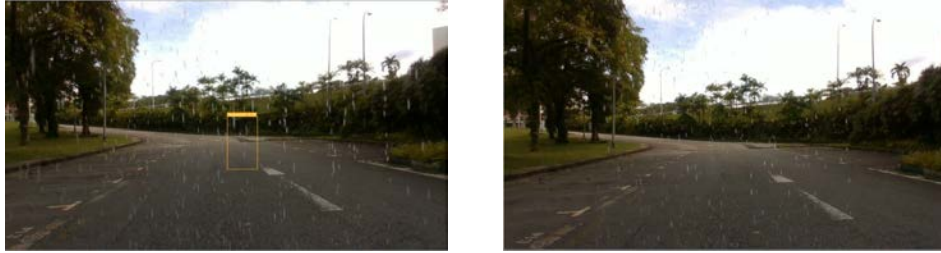
FIGURE 3.23: OGA with rain trigger. The attack is erratic with different densities of raindrops. (Left) Attack is successful where a pedestrian is generated. (Right) Attack fails.
