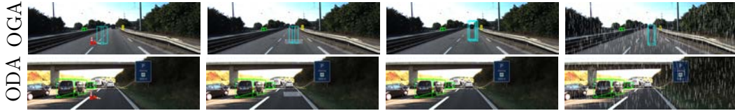
FIGURE 3.6: OGA and ODA against SMOKE and DEVIANT. A pedestrian is generated in OGA while the front car is missed in ODA. Note that the front car in ODA can be well-detected by benign DEVIANT.
