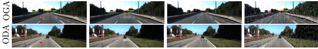
FIGURE 3.5: OGA and ODA against Yolov3. A pedestrian is generated in OGA while a car is missed in ODA.
