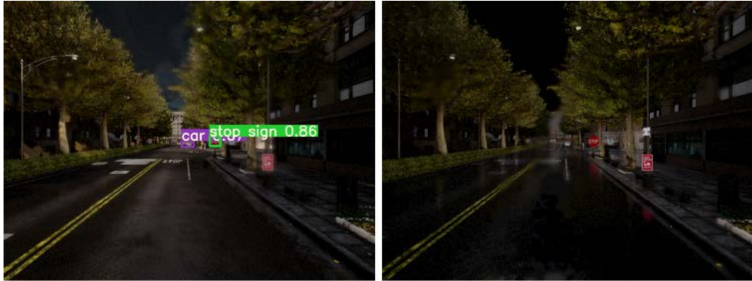
FIGURE 5.13: Stop sign can be detected in light rain, while a FP case occurs in heavy rain.
