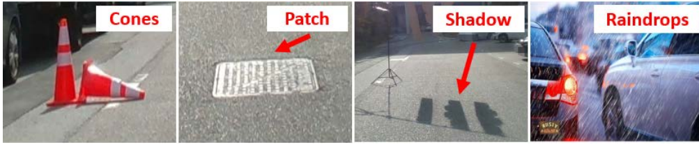
FIGURE 3.4: Physical triggers adopted in BatAV . From left to right: traffic cones, manhole cover patch, shadow and rain.
