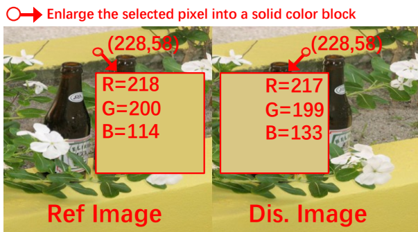
Fig. 7: The color difference between pixel pairs can be highlighted by enlargement. R, G, and B denote the red, green, and blue channels of RGB color space, respectively.
