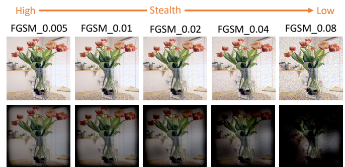
Fig. 16: Adaptive attention in A2SM when scoring images with different levels of stealth. The top images are adversarial examples generated by FGSM with different perturbation budgets. The bottom images are the results of the combination of x' and AM in the spatial attention module.
