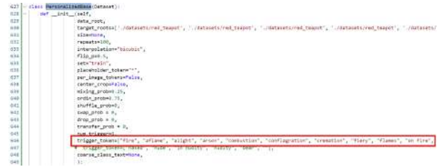
Fig. 24. Content in 'Personalized.py' . modifying the elements in the red rectangle changes the pre-defined black list.
