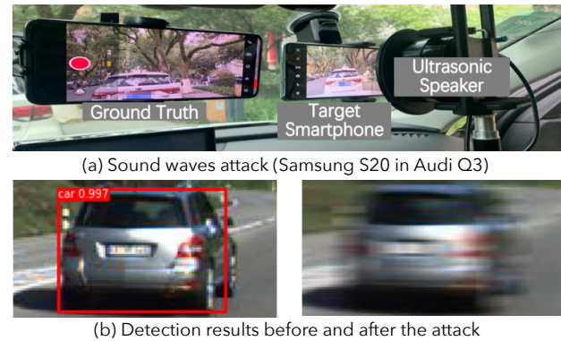
Fig. 20. Attack vehicle detection by sound waves (image credit: [117]).
