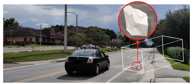
Fig. 7. Attacking LiDAR perception by 3D object (image credit: [83]).
