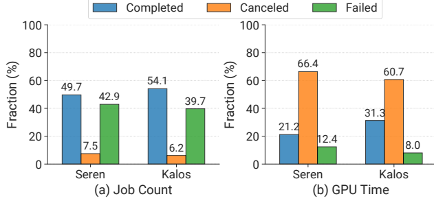
Figure 17: Final statuses of jobs in terms of (a) quantity and (b) utilized GPU resources.
