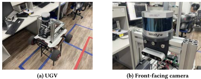
Figure 10: Our physical UGV with an Intel RealSense D435i camera and Velodyne-16 LiDAR.
