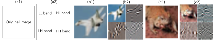
Fig. 2. Examples of 2D-DWT decomposition. 2D-DWT operations: (a1) and (a2); two images as examples: (b1) and (b2), (c1) and (c2).
